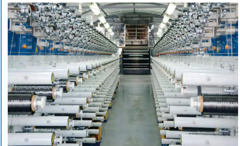
© Production Line of T1000 Carbon Fiber of Zhongfu Shenyang
